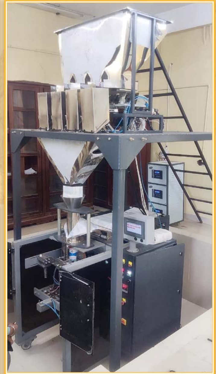
High throughput seed processing - Modern processing and packing machine established (2023)
